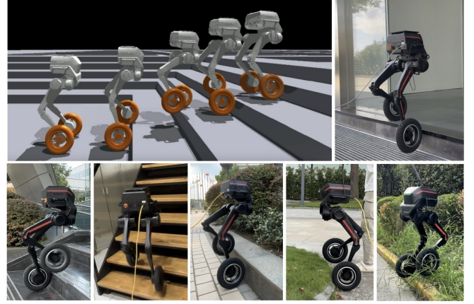
Fig. 1. We have developed a contact-triggered blind climbing control policy that works for wheeled-legged robots of various tire sizes, enabling them to conquer a variety of challenging terrains.
